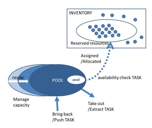
The Push TASK increases the size of the Pool by adding resources to the Middle B assignment Pool according to the request of Middle B.
